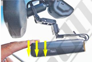
4 - If the RD is too close to the bottom of the mirror, You may access the buttons on top of the RD by gently pushing downward on the front of the RD with one finger and push the desired button with another finger. Then allow the RD to return to it's original position by gently letting it spring upward. When accessing the buttons, be sure to push the RD downward just enough for your finger to fit between the RD and mirror. Do not push down more than what is needed.
